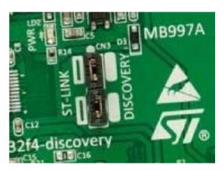
Note that pin 1 of the 6-pin SWD interface on CN2 of the Discovery board only **detects** the voltage of the target. Thus the most foolproof method of flashing is to connect a mini USB cable to the 407v board and set the power switch to USB. This ensures that the board is always powered up when programming. After the bootloader is burned in, the 407v board can be installed in the wCore PCB through the two 2\*25 headers.
