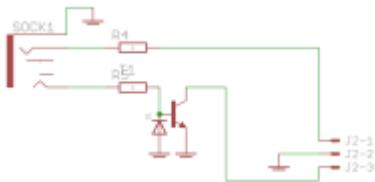
To use the socket for another purpose (audio input or output?), feel free to omit the diode and transistor, and to bridge the collector and base pins.
