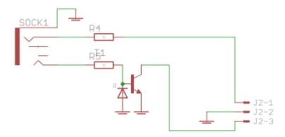
To use the socket for another purpose (audio input or output?), feel free to omit the diode and transistor, and to bridge the collector and base pins.
