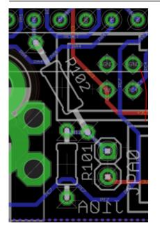
This jumper replaces the "bootloader" functionality of the Discovery board's blue button. It could be wired to an external panel control if needed.
