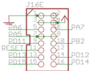
The original J16 functionality is preserved, but extra pins are available on a IDC16 header. These include the Reset signal and pins normally controlling LEDs. This header is normally connected to the [RES-SD module](#).
