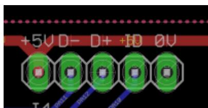
This header supplies +5V, 0V, USB data and the ID state. Normally it will be connected to the [USB module](#) by a short cable.
