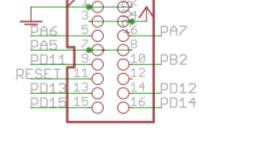
The original J16 functionality is preserved, but extra pins are available on an IDC16 header. These include the Reset signal and pins normally controlling LEDs. This header is normally connected to the RES-SD module.
