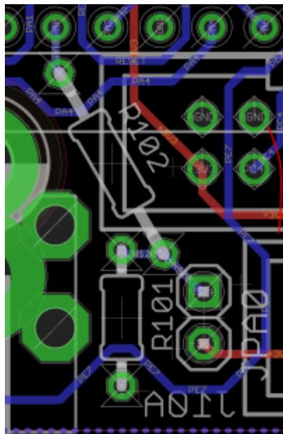
This jumper replaces the “bootloader” functionality of the Discovery board's blue button. It could be wired to an external panel control if needed.
