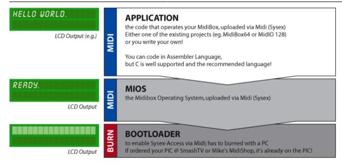
MIOS is the operating system of the microchip. It can be uploaded by SysEx (via MIDI) thanks to a bootloader, a special software that is already burned onto the chip if you order at SmashTV's or Mike's Shop.
