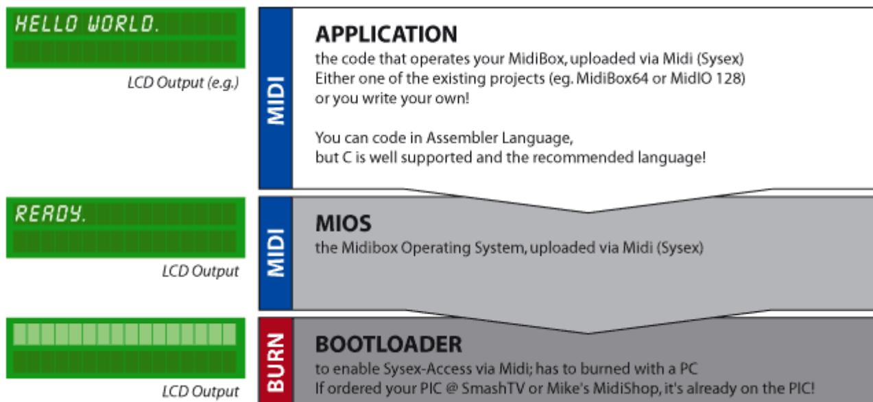
**MIOS** is the operating system of the microchip. It can be uploaded by SysEx (via MIDI) thanks to a **bootstrap** loader, a special software that is already burned onto the chip if you order at SmashTV's or Mike's Shop.
