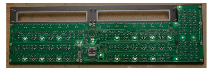
Now is a good time to do a "fit test" of the PCB and panel with temporarily mounted studs.
