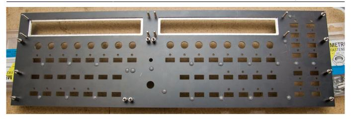
Do a final check that the switches (if you have them inserted) are properly inserted into the PCBs, and that the spacers are mounted in the right positions.
