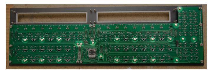
Now is a good time to do a "fit test" of the PCB and panel with temporarily mounted studs.
