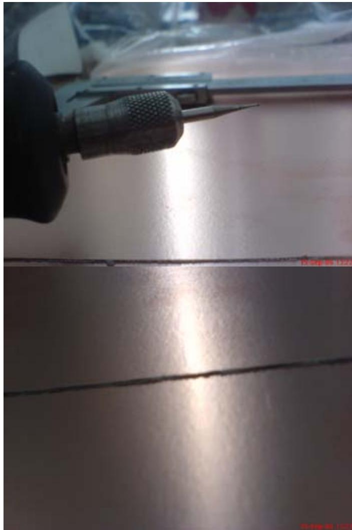
Drilling the new PCB using the old PCB as template. Doing so you achieve a perfect fit of your PCB into the unit. Don't forget to drill the mounting holes too. I am using clamps to keep the two boards aligned during the process
