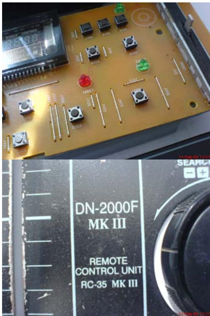
After that I desoldered the PCB to have a template for making new ones. This was done with the help of a desoldering pump. The pushbuttons, the leds and the jog/shuttle wheel have been desoldered.
