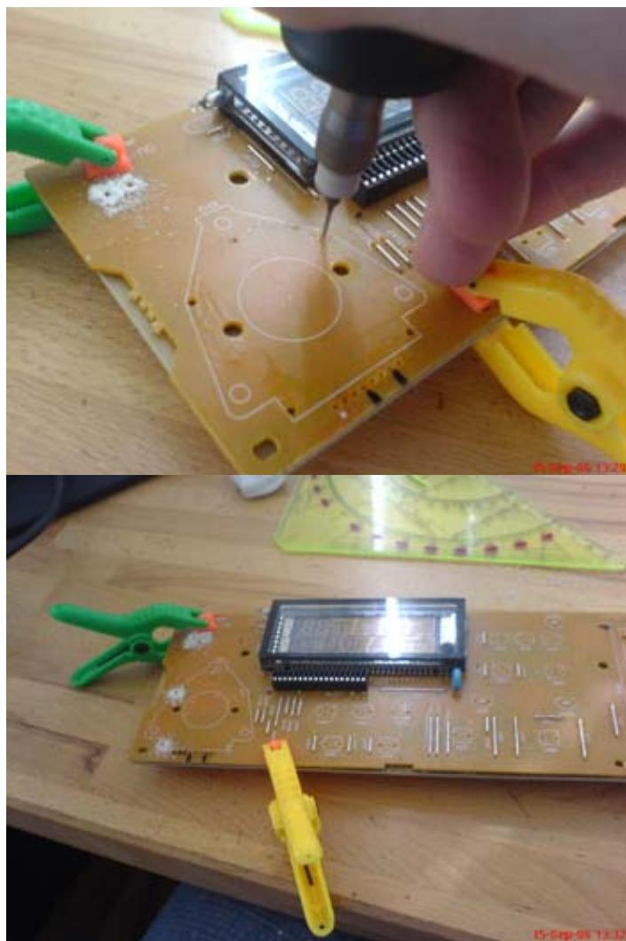
Afterwards I milled new soldering pads using my dremel tool again. One pin from each pushbutton is insulated from the rest of the board (which acts as ground) this way.
