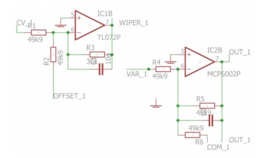
The circuit is a very simple series of two inverting amplifiers per channel. The first is a TL072 powered from +12/-12V, while the second is an MCP6002 powered from 3v3/0V (ground). It's possible to preset the ranges (see below) but it's probably more useful to use the associated Control Board.
