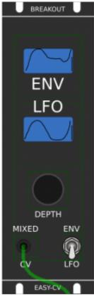
**Envelope Scope:** show the ENV-Waveform or the Mixed-CV-Output-Waveform (when Switch is in LFO Mode)
