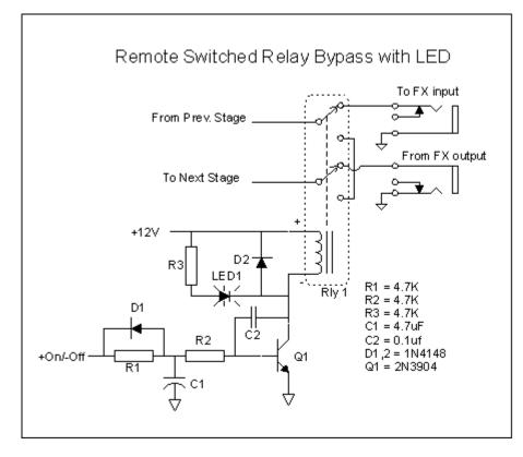
"The neat way to defeat the clicks is to slow down the change in voltage across the inductor. The circuit at left does that. An
