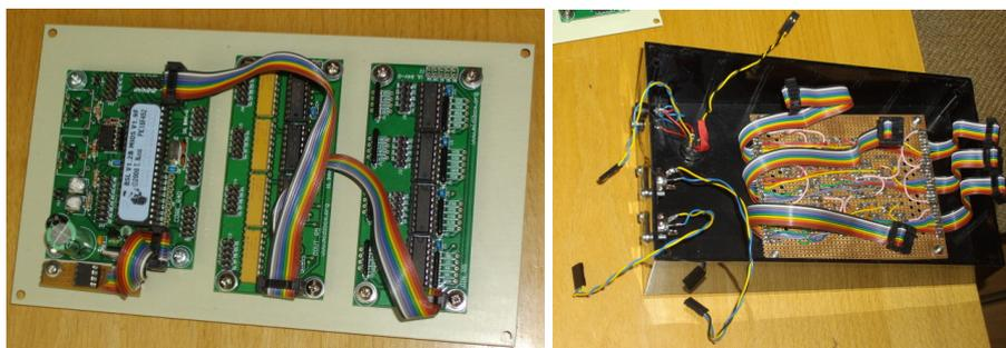
The board for the buttons is realized with a labour board with copper rows:
