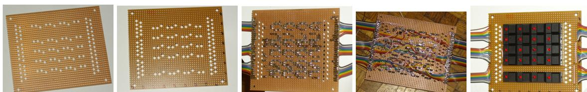
On one side you have the DIN ribbon cables, on the other the DOUT's. On each ribbon cable you have eight of them, one track is a ground. One track stays unused. The connections must match the assignment of the DIL pin-headers for the connection to the DIN/DOUT boards. Note that DOUT's are counted backward for each SR/plug/ribbon cable. See [this](#) page for more information about the issue.
