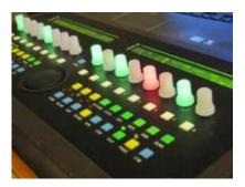
Since I used a custom design I put all the buttons/leds/encoders on a standard 0,1 inch vectorboard. I had to cut a hole into it because I had to fit the data wheel in between.
