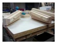
The trick with the baseplate is to cut a gap along the lower bound of the frame parts.
