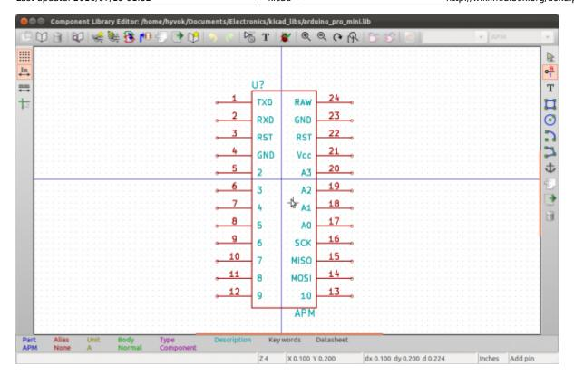
• Then you have to create a Schematic, which is the Conceptual Drawing of your electronic design. It's how components are connected together.
