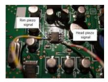
Here the signals are centered around 2.5 volts. After a few experiments I found that these signals are too weak to be fed directly into the LPCXpresso board's ADC inputs, they need some gain.
