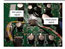
Here the signals are centered around 2.5 volts. After a few experiments I found that these signals are too weak to be fed directly into the LPCXpresso board's ADC inputs, they need some gain.
