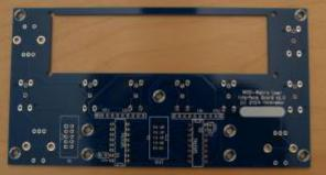
The total size of the PCB is 150mm x 80mm.
