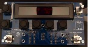
A second generation PCB as pictured above has been ordered and tested to work. This PCB can also be used with other projects involving an SCS, e.g. the MIDIbox NG. Both, my favourite switches from Marguardt (6425 series), as well as the E-Switch TL1100 series (see e.g. MB SEQv4) can be used.
