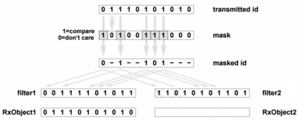
Left filter allows the packet to go into the buffer, right filter rejects it.
