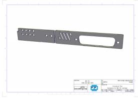
It's a 1.5mm thick aluminum plate. There's **two part** which have to be separated
