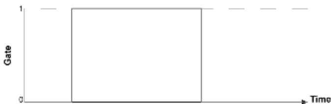
Gate Stay active option maintain the Gate High and allow to dig in Amplitude(useful when depth velocity or envelope are negatives).
