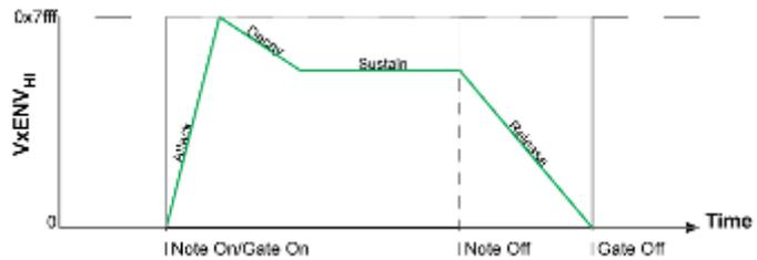
Envelope to Amplitude Enabler in Vx Mode Controller:
