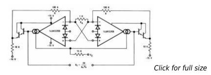
A floating VCR where each "end" of the "resistor" may be at any voltage within the output voltage range of the LM13700.
