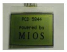
PCD8544 LCDs are very small and providing only a resolution of 84×48.
