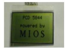
PCD8544 LCDs are very small and providing only a resolution of 84×48.
