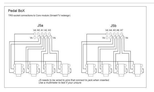
When inserting/removing a jack, make sure the control voltage = 0 (pedal off). Or you will pass
