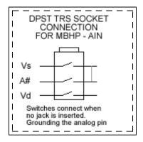
I use normalising (DPST) 6.5mm TRS Sockets. Tip = +5 (vd) Ring = CV (A#) Sleeve = Ground (vs)
