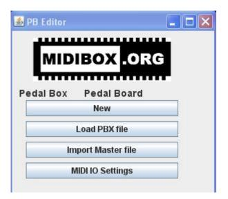
**New** - Opens a new Master Bankstick Window with default data loaded. This can be modified to suit your rig.
