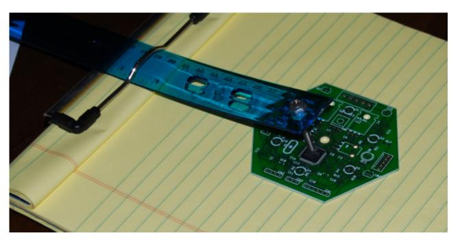
That chip will stay put easily while soldering, and the ruler puts only a LIGHT pressure on the chip, so nothing gets damaged. No, that's not a MBMixer board, those have not arrived yet. (But it is a PIC18F458, alternate core, anyone?)
