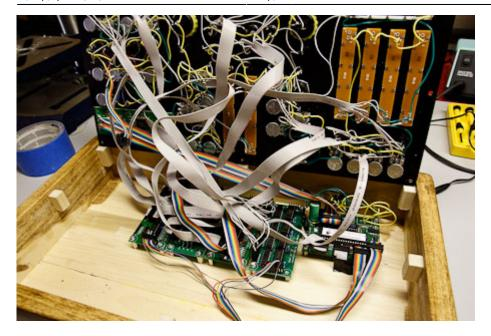
**Wiring the Panel:** Now comes the tedious and time consuming part of the build, wiring the front panel. For the most part, the PDF diagrams on the ucapps site that accompany each module are the keys to understanding the wiring sequence. I'm using ribbon cable, as it will be easy to attach to the modules, and keeps the overal spaghetti-ness of the panel down considerably.
