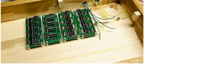
The shot above shows the module PCB's attached, awaiting the core module being hooked up to midi wiring and the power input.
