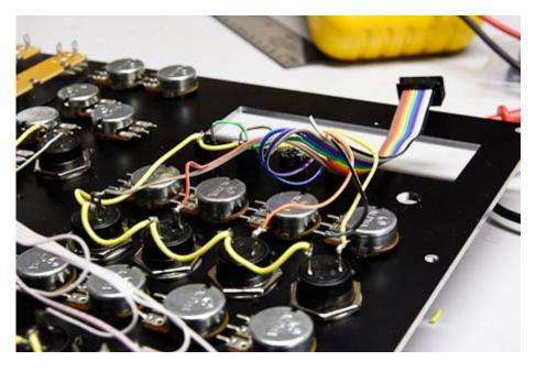
Here's a detail shot of the grounding sequence for the buttons. The black wire on the ribbon cable is connected to the VS pin on the DIN board. The rest go to their individual buttons. The black cable is then daisy-chained from one button to the next (via the yellow, thicker wire) until all of the buttons have been grounded.
