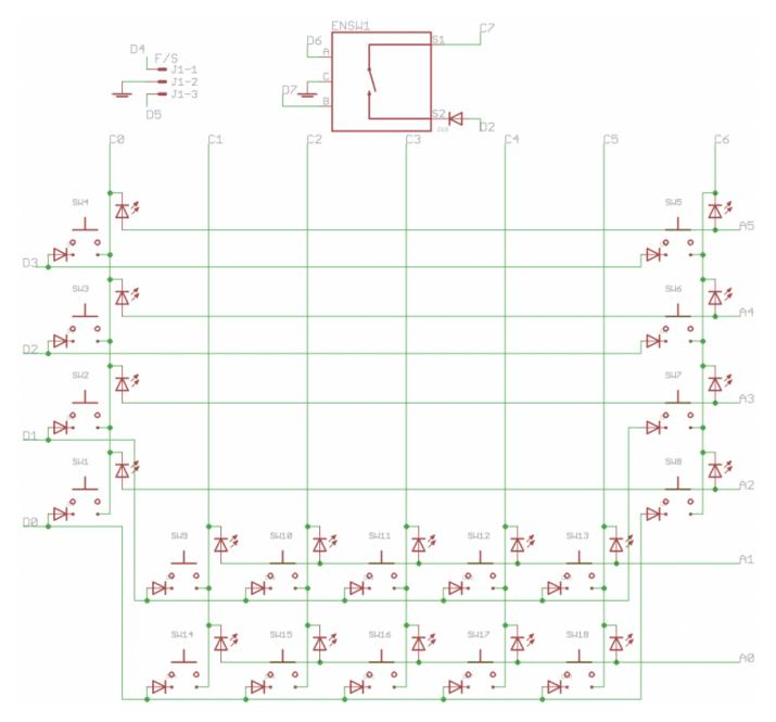
Note the encoder connected to pins D7 and D6, and header J1 connected directly to D5 and D4. All of the cathode rows are used, even C7 just for the encoder push switch.
