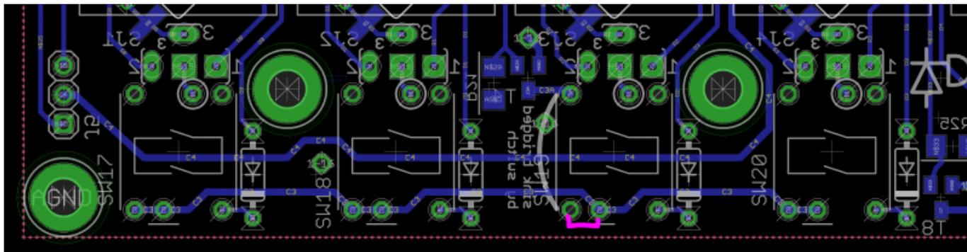
Ghosting. As seems common with these kinds of matrices, there is some unwanted lighting of LEDs. This is most apparent when trying to light up the bottom row of MEC switch LEDs, as the resistive path to the Superflux LED is lower and thus glows unintentionally. This can be overcome somewhat by stacking BAT54 Schottky diodes on top of the BC18 transistors. Later revisions will have more elegant mounting.
