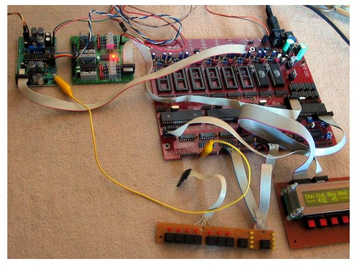
My prototyping setup, a MBSID V2 (MB-6582 base PCB) with 6581 SIDs and an AOUT\_NG.
