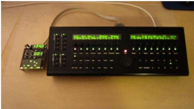
In my MIDIbox SEQv4, the TPD is sitting below Wilba's control surface panel, and to the left of my [16x4 Button LED Matrix board](#). This makes for a nice and clean user interface and can be easily built into a 19" / 17" wide case.
