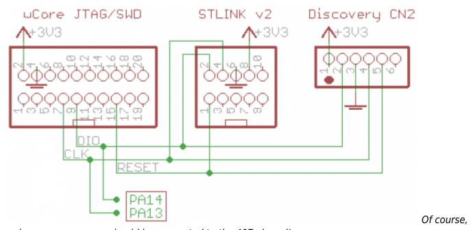
only one programmer should be connected to the 407v board!
