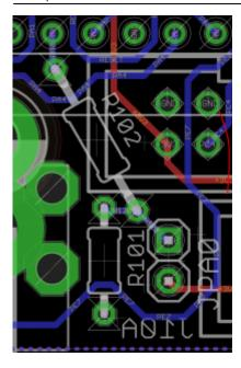
This jumper replaces the "bootloader" functionality of the Discovery board's blue button. It could be wired to an external panel control if needed.
