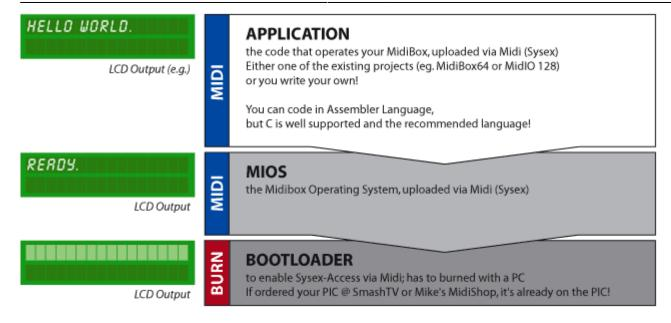
MIOS is the operating system of the microchip. It can be uploaded by SysEx (via MIDI) thanks to a bootstrap loader, a special software that is already burned onto the chip if you order at SmashTV's or Mike's Shop.
