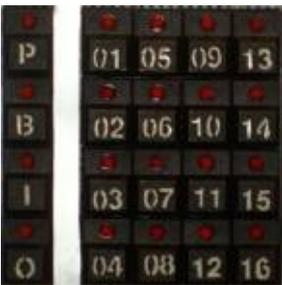
The User-Interface panel consists of 20 buttons. There are 4 "screen-buttons" and 16 "value-buttons". Each button has a associated LED. If you push a screen button, the device will switch to this screen, the value LED's will show the selected value(s) for this screen. If you push a value-button, this value will be selected or de-selected.
