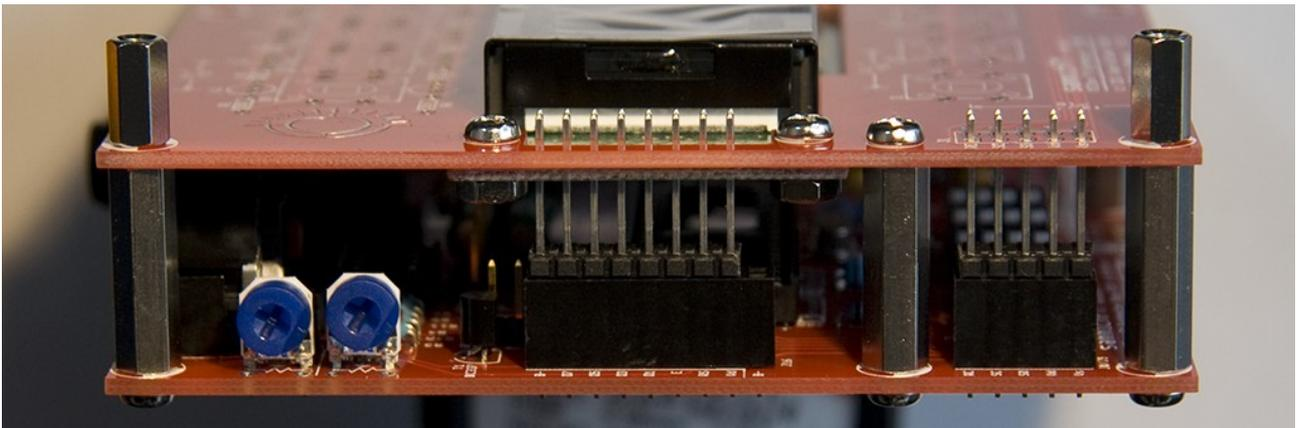
**Step 7.6:** Solder two diagonally opposite pins on each header on the top side, ensuring female header is flat against base PCB.
