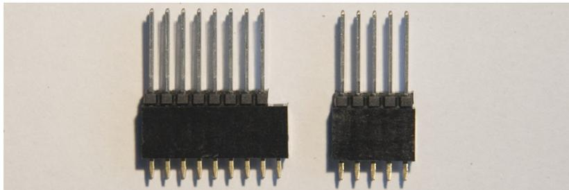
*Note: depending on the LCD type, the 16 pin male header goes into the “upper” or “lower” 16 pins of the 18 pin female header. Most of the time it will be the “upper” 16 pins, as shown by the white outline on the base PCB. As far as I know, only the Optrex STEP LCDs require it in the “lower” 16 pins, because the backlight pins are at the other end of the header.*
