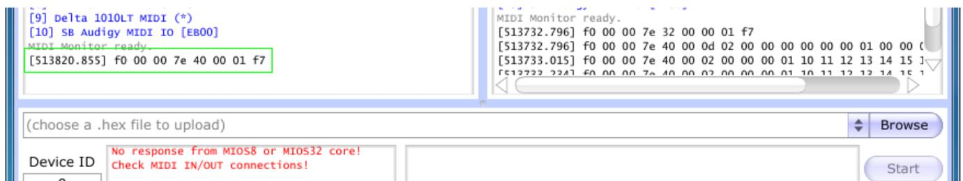
This is because the PIC18F4685 has already been burned with MIOS 1.9g. If you get this message, then you know the PIC is working and MIDI Out is working. MIOS installation can also be confirmed by the LCD showing the MIOS startup message.
