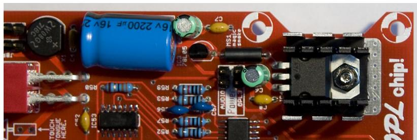
**Step 5.3:** Place big heatsink onto PCB
