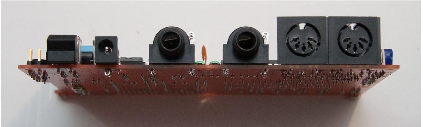
Solder only *one pin* of each socket to hold it in place, then you can check for correct alignment before soldering the other pins.
