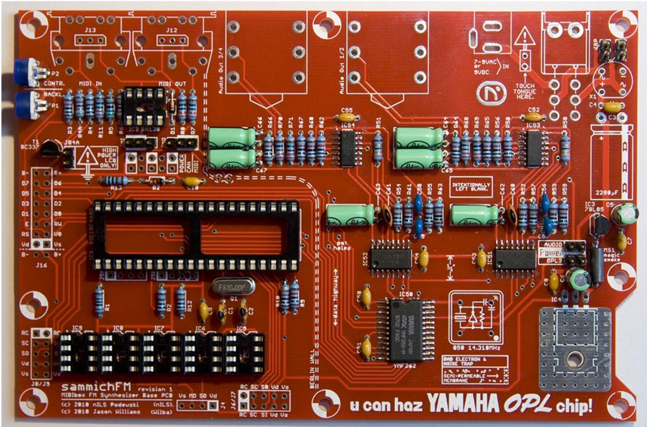
Electrolytic capacitors must be oriented correctly. The lead identified by a black stripe (with “-” inside) is the negative lead. The *other* lead must go in the positive pad, identified with a “+” on the part outline.
