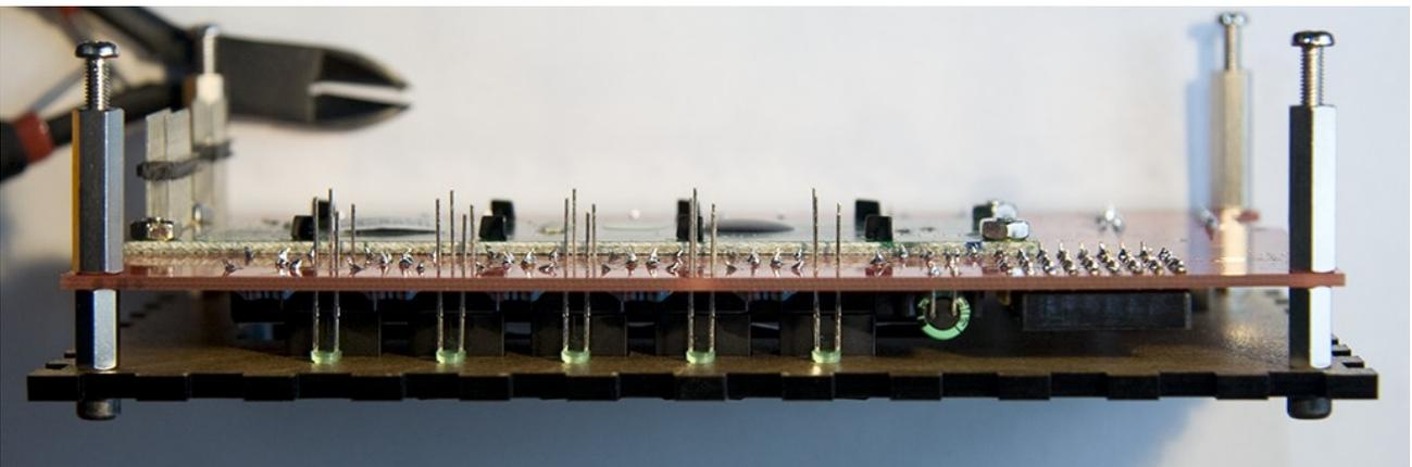
**Step 3.6:** Look underneath at the LEDs and check they all protrude the same amount. If any do not, it could be that a LED is stuck because the hole is slightly smaller or the LED is slightly bigger. Disassemble PCB and panel and check that LED individually. It is possible that a LED has a little bit of excess plastic from molding imperfections, which can be scraped away using a craft knife.
