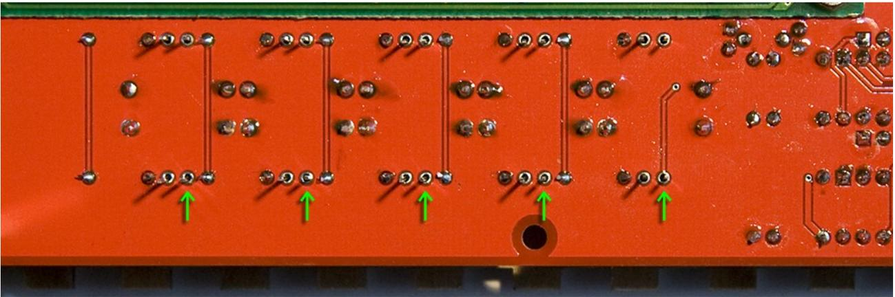
**Step 3.8:** Look underneath at the LEDs and check they all protrude the same amount. If not, heat up a joint and push down on the longer lead (there's a reason I told you to solder the shorter lead first!)
