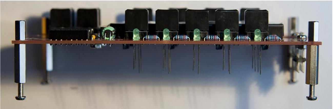
**Step 3.4:** Attach top panel to PCB using black screws. Check alignment by looking at the switch caps.
