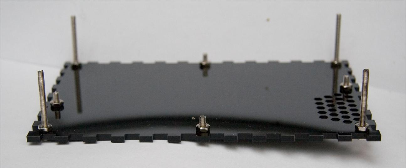
Put the 32mm and 9mm screws into the base panel from the bottom. The 32mm screws go in the corners. Add the nuts and tighten firmly using screwdriver and long-nose pliers.
