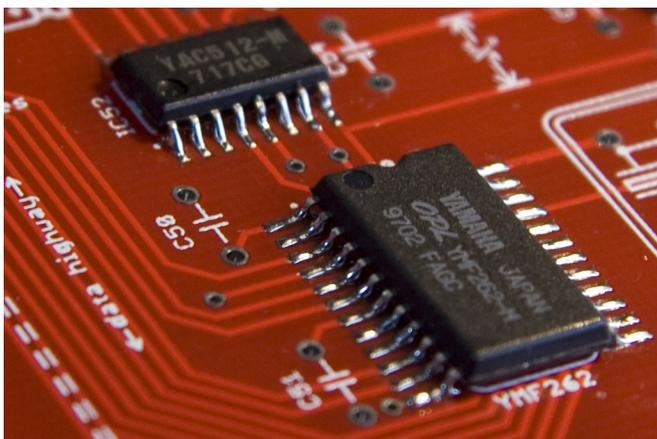
*Here is an example of the YMF262 and YAC512 soldered with “good” solder joints, IMHO. Observe how the solder fills the space behind the pin, between the pin and the pad, and a little bit stuck to the inside bend on the top of the pin. This may be more solder than what you might see in a factory assembled PCB, because they use tiny amounts of solder paste and cook it in an oven. You could remove some of this excess with solder wick, but it's not necessary.*
