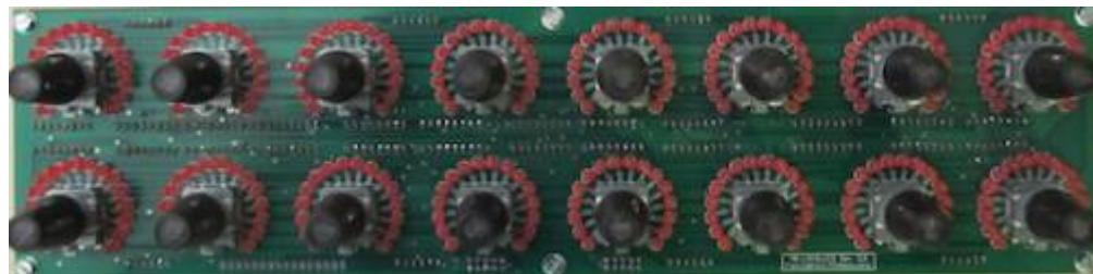
Up to 32 free assignable rotary encoder functions with support for LED rings are available. The encoders have to be connected to a MBHP\_DIN module, the LED rings to four shift registers of a MBHP\_DOUT module.
