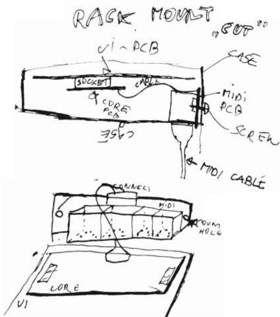
Showing a 10x4cm sized Core32 plugged into a 10x10cm UI-PCB also a midiport-solution is shown, where a midiPCB is fabricated on the core PCB but with the possibility to break it down, the optocouplers diodes and Resistors for the Midiports are on the Core PCB, so the Midi-IO pcb can be small as possible, so we achieve a small Project (small case, small ui...)
