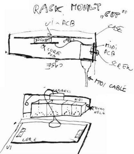
Showing a 10x4cm sized Core32 plugged into a 10x10cm UI-PCB also a midiport-solution is shown, where a midiPCB is fabricated on the core PCB but with the possibility to break it down, the optocouplers diodes and Resistors for the Midipoorts are on the Core PCB, so the Midi-IO pcb can be small as possible, so we achieve a small Project (small case, small ui...)
