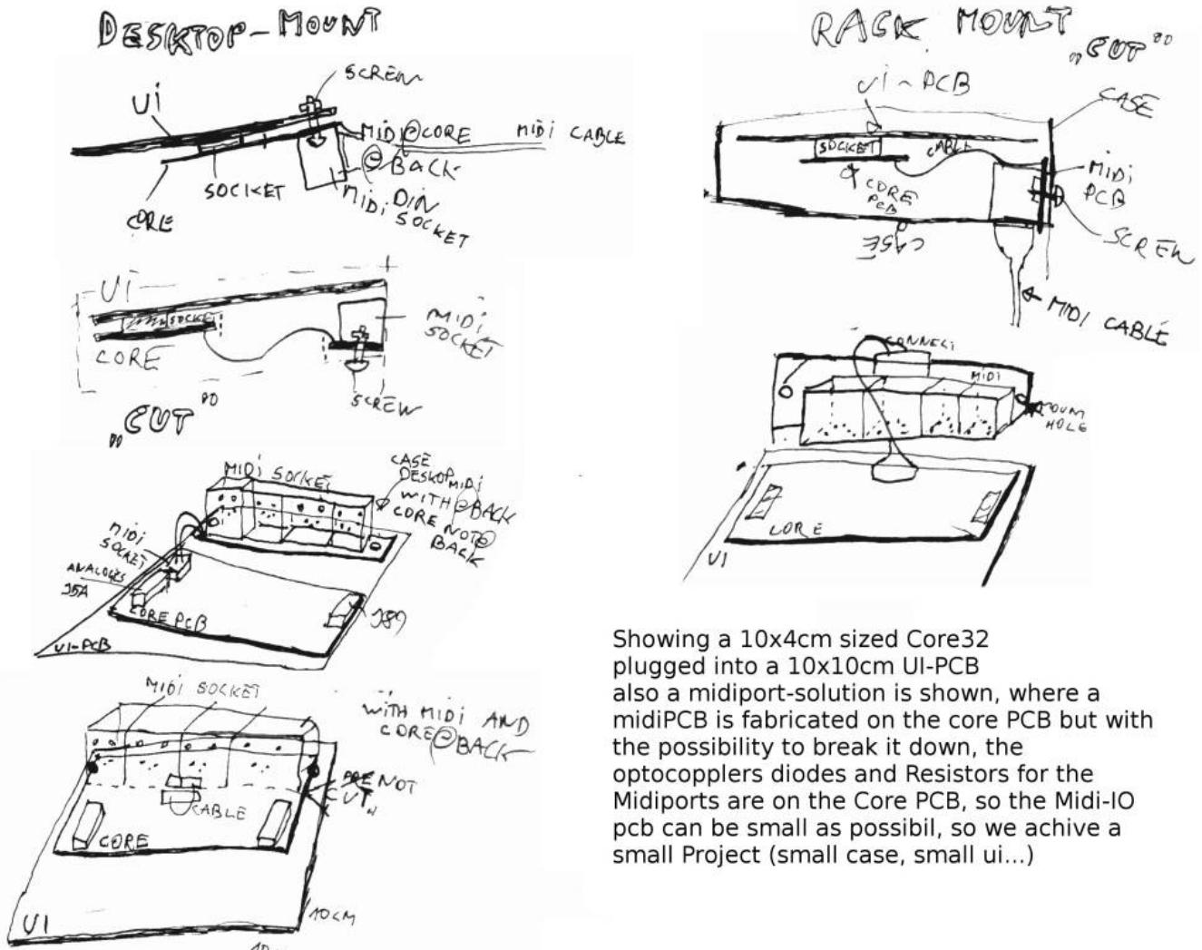
Showing a 10x4cm sized Core32 plugged into a 10x10cm UI-PCB also a midiport-solution is shown, where a midiPCB is fabricated on the core PCB but with the possibility to break it down, the optocouplers diodes and Resistors for the Midiports are on the Core PCB, so the Midi-IO pcb can be small as possible, so we achive a small Project (small case, small ui...)
