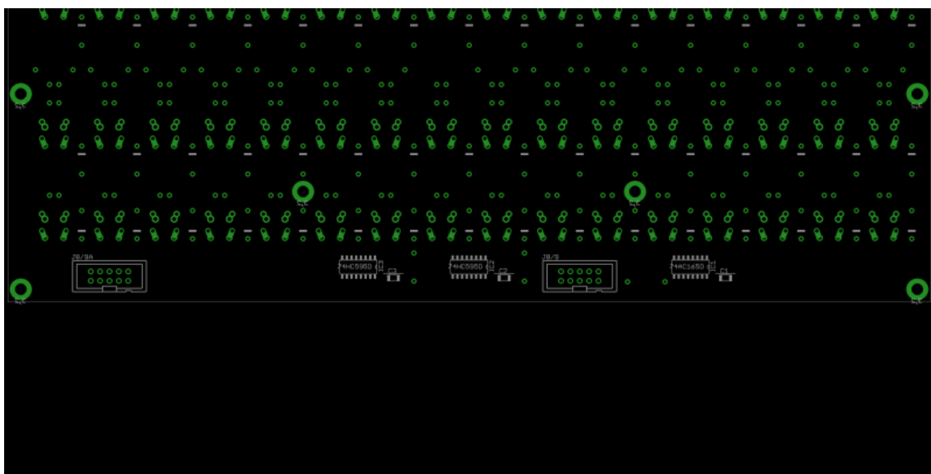
Rear placement of ICs (ignore the "AC" package, the correct CMOS family is 74HC165)
