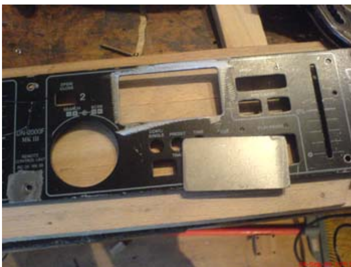
Partly finished after bondding and sanding.
